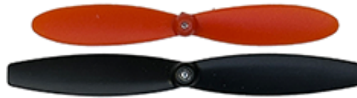
Figure 7: Dromida Hovershot (top) and Parrot Mambo (bottom) propellers.
