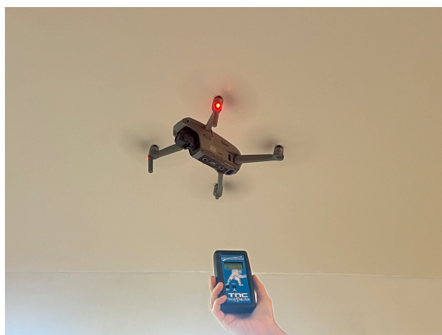
Figure 36: Measurement of propeller RPM while in flight using a handheld tachometer.
