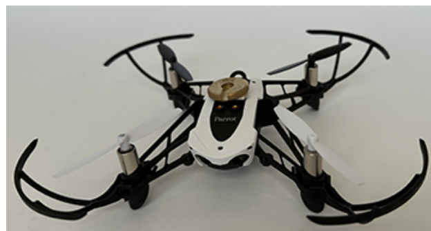
Figure 37: Example loading of additional weight on the Parrot Mambo.
