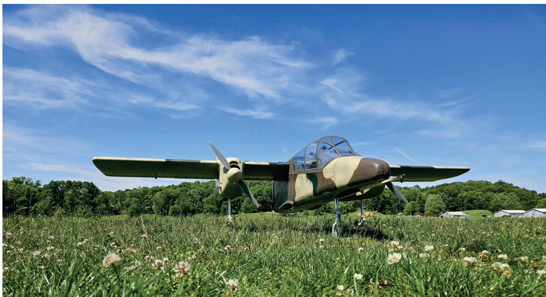
Figure 1. Flight-ready Hangar 9 OV-10 Bronco 30cc UAV testbed prepared for initial flight evaluation. The aircraft was configured with the stock electric twin-engine configuration and prepared without the full sensor payload installed.
