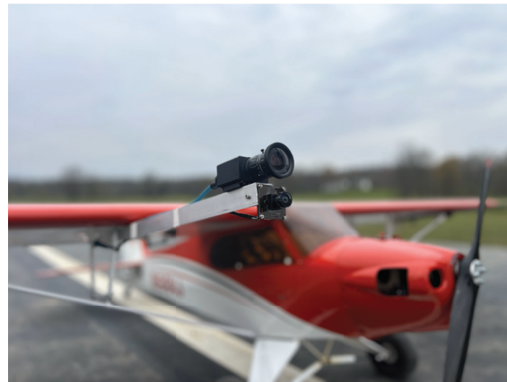
Figure 4. The single frame camera and an event camera used for data collection on the original experimentation UAV. 25
