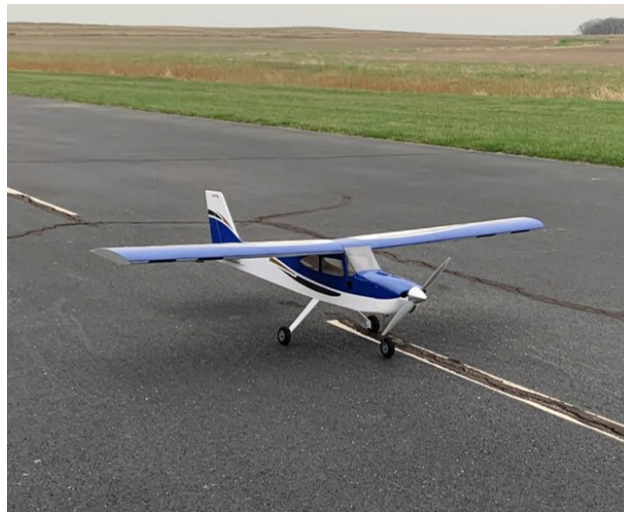
Fig. 7 The flight-ready, baseline 90.5 in (2.3 m) wingspan Avistar 30 unmanned aircraft.
